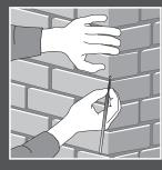
F. Once the filler paste is dry, paint the joint with Panespol special paint. Finish off by applying Panespol's ferrous oxide coating to give a perfect result.
