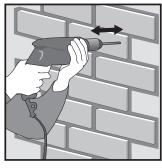
**3.** Fit the panel to the wall and drill through the panel directly into the wall using a 6mm drill bit, Put the screw into the wall-plug and introduce both into the hole in the panel. Push and screw them in until the panel is securely fixed (e.g. "Fisher" 6mm wall plugs and 4,5 x 40 screws are recommended). Use as many screws per panel as are needed.
