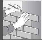
**B.** From this line, mark a parallel line away from the wall at a distance equal to double the thickness of the panel - between 2 and 4 cm depending on the model. (This will be the outside line of the cut)
